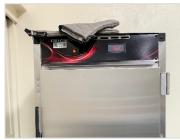
Step 5 Load light trays in the upper section of the hot holding unit.
